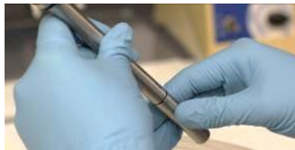
4. While holding the probe slanted, screw the probe back into the cap. Some of the solution should spill out.
