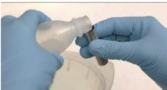
3. Fill ½ to ¾ with new electrolyte solution.
